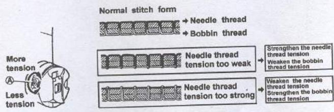
Thread tension should be determined in accordance with the stitches obtained by adjusting the tension of the bobbin thread and needle tension (Fig. 12).
