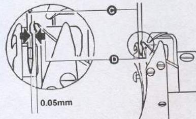
When lifting the needle bar from its lowest position of the stroke to the distance A, the hook point D of the bobbin should align with the center line of the needle and be 1.0 – 1.5 mm above the upper end of the needle eye. (Fig. 15)
