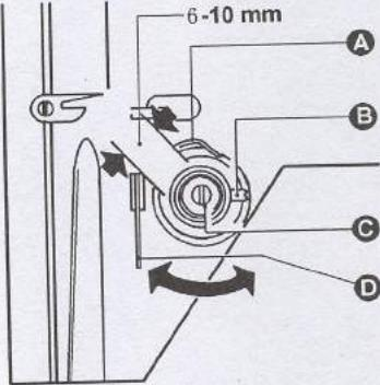
The tension of the needle thread: to be adjusted by turning the thumb nut.
