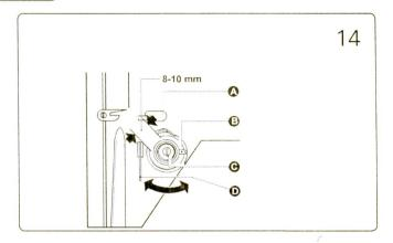
The tension of the needle thread: to be adjusted by turning the thumb nut.
