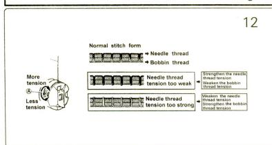
Thread tension should be determined in accordance with the stitches obtained by adjusting the tension of the bobbin thread and needle tension (Fig. 12).
